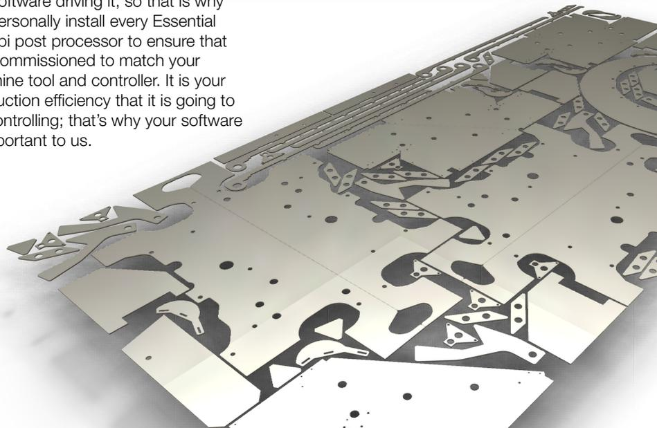
Essential Combi intelligently applies the profile tool paths automatically at the nesting stage for profile machines to maintain the quality and integrity of your parts, whilst also optimising the cutting sequence and ensuring cutting head safety, thus enabling the machine tool to perform to its optimum potential
